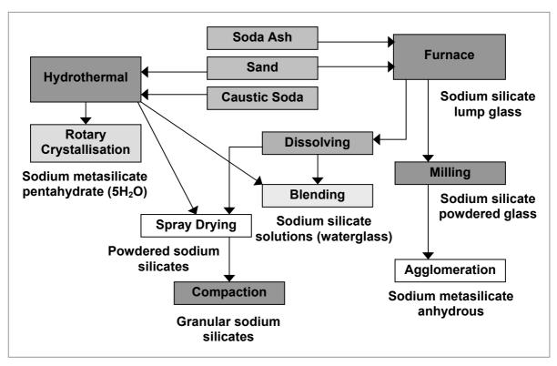
**DIAGRAM 6:** Soluble silicates manufacturing process
