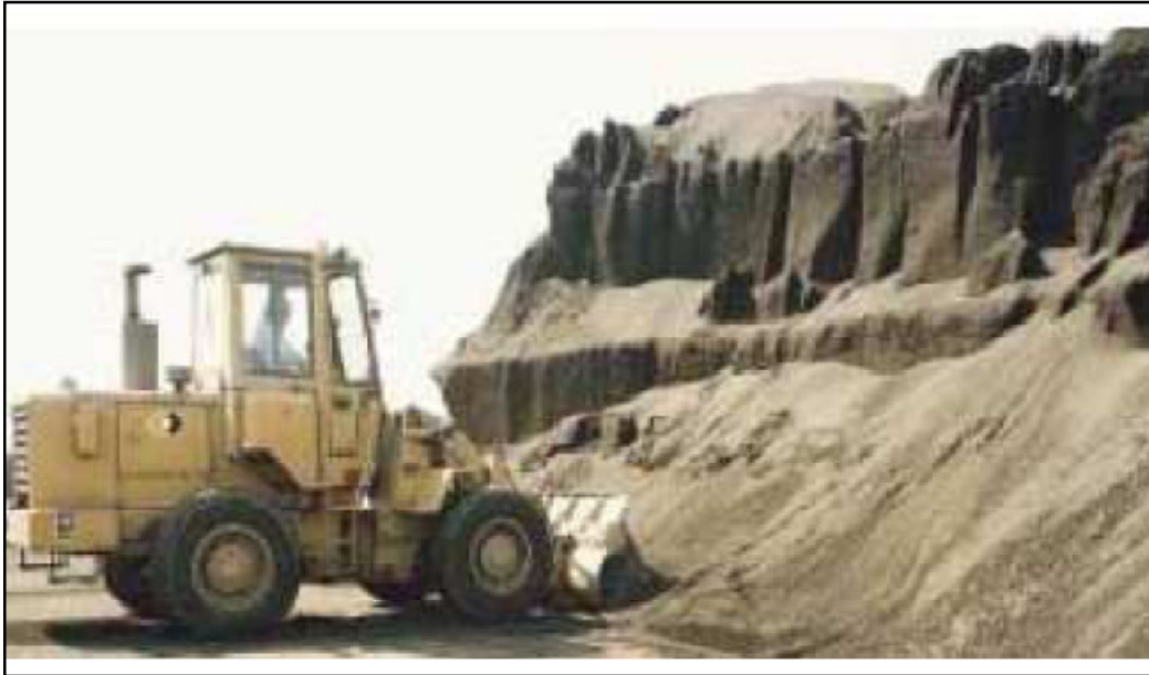
Figure 5: Mechanical mining employing front end loaders (Source: Namakwa Sands)
