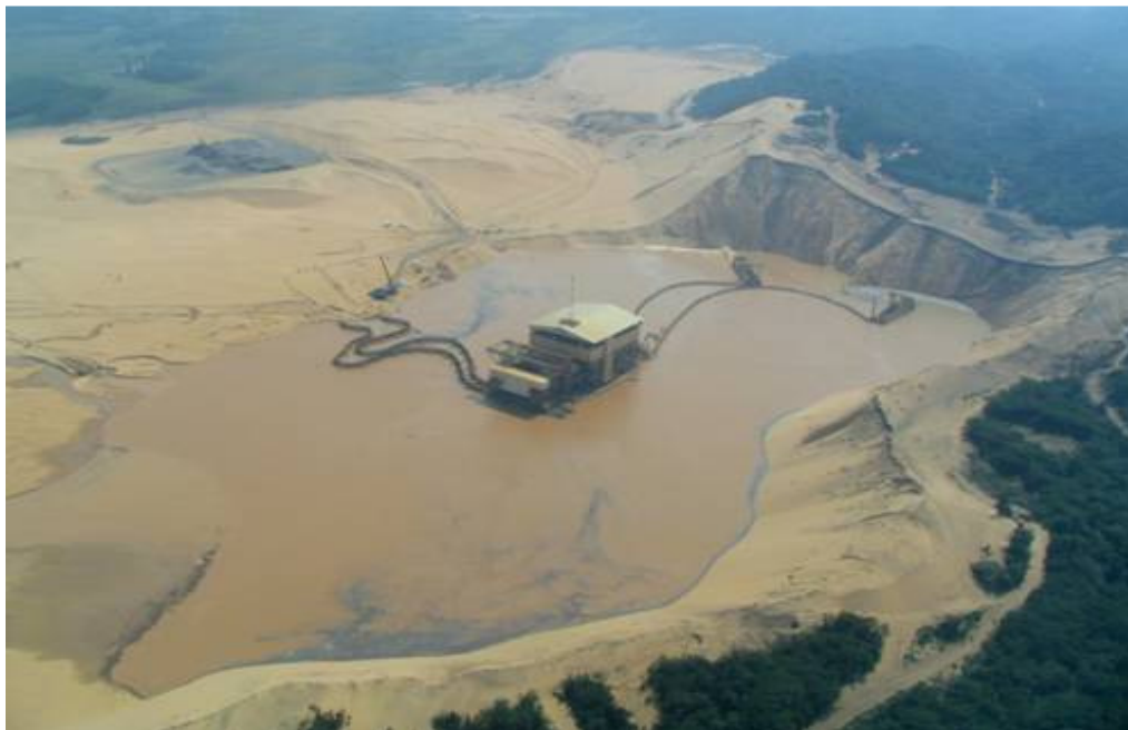
Figure 6: Dredge mining employing a floating dredger
