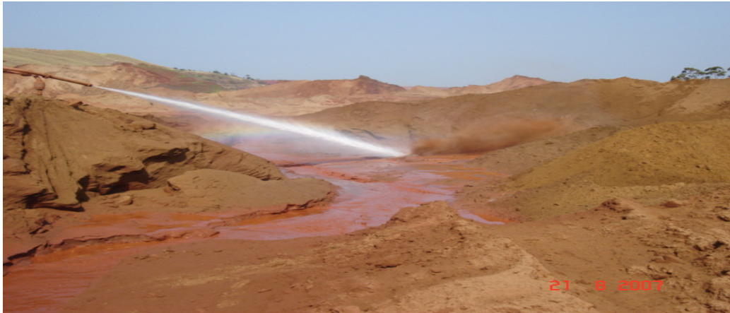
Figure 4: Monitoring mining employing water Guns
