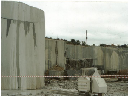
Fig 3: Diamond wire-cutter in operation
