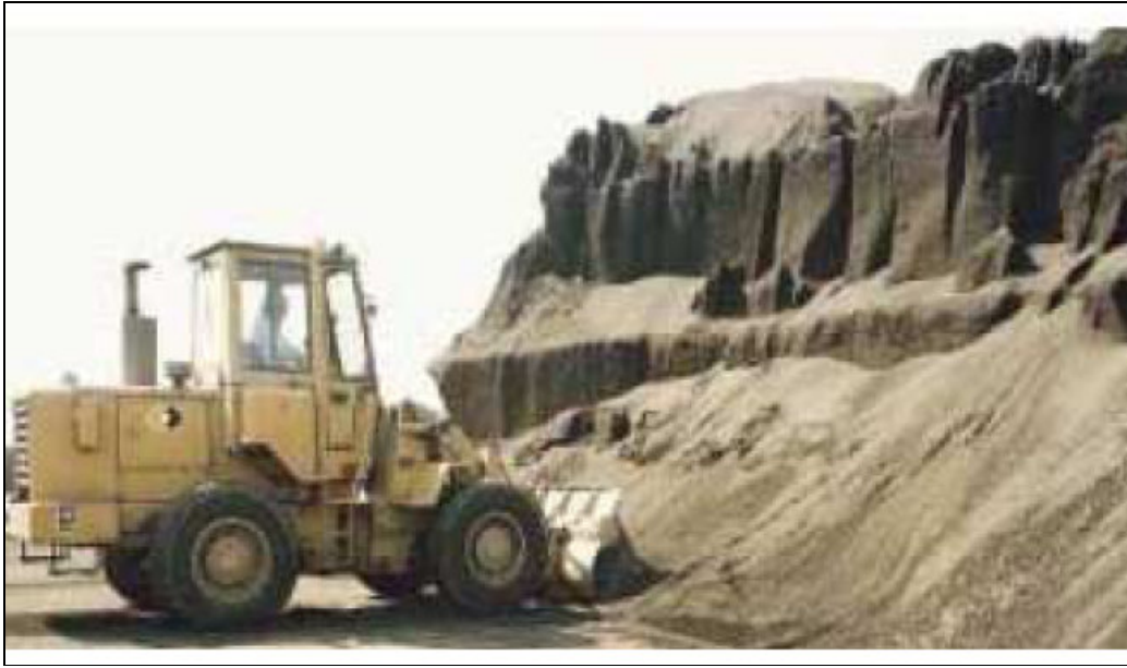
Figure 5: Mechanical mining employing front end loaders (Source: Namakwa Sands)
