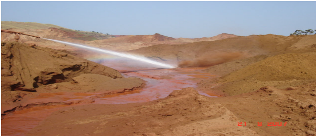
Figure 4: Monitoring mining employing water Guns
