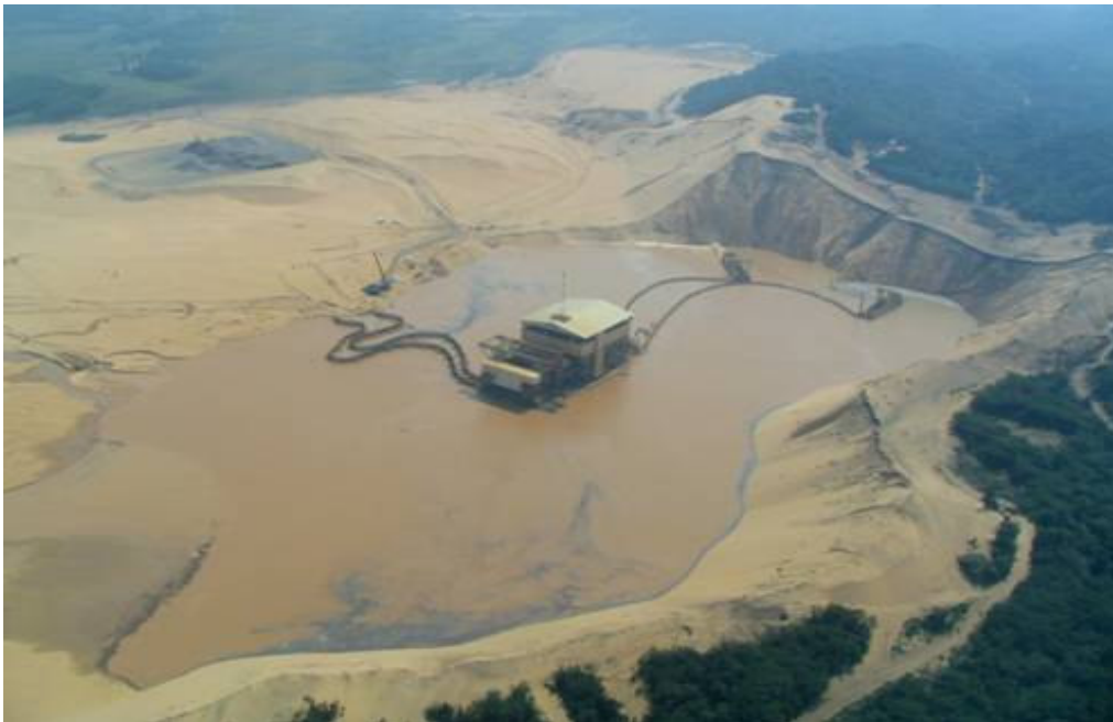
Figure 6: Dredge mining employing a floating dredger
