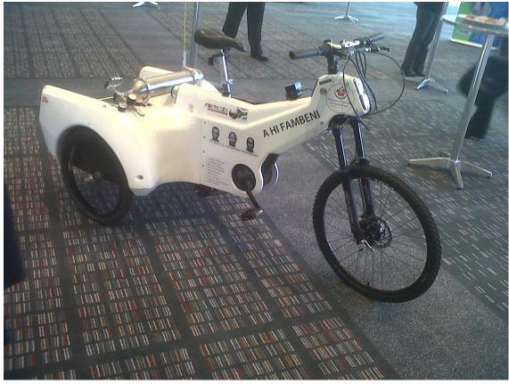
FIGURE 4: A HYDROGEN FUEL CELL POWERED BICYCLE BUILT BY TUT STUDENTS IN PRETORIA.
