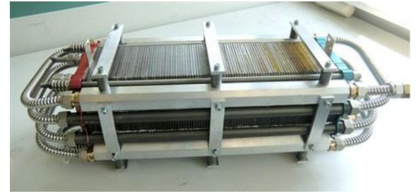
FIGURE 3: THE HIGH TEMPERATURE PEM FUEL CELL, ASSEMBLED BY HYSA SYSTEMS.
