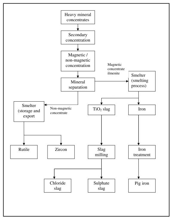
Figure 2: Basic flow diagram of titanium-bearing minerals processing
