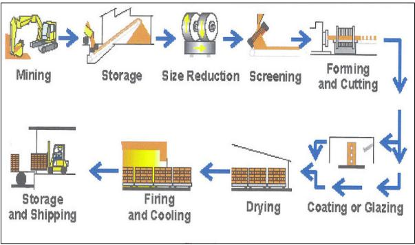
Figure 2: Basic brick making process
